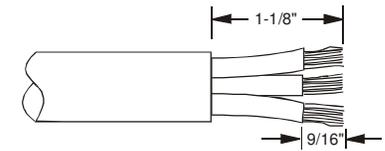
**4. Assembly:** Insert all the wires into the proper terminal pockets. The green wire must go into the terminal with the green colored screw (also marked "GR"). The white wire must go into the terminal with the silver colored terminal screw (on 125V and 277V devices only) The black wire must go into the terminal with a brass, or black colored screw.
