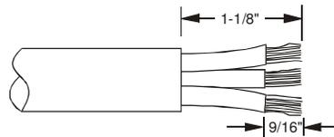
**4. Assembly:** Insert all the wires into the proper terminal pockets. The green wire must go into the terminal with the green colored screw (also marked "GR"). The white wire must go into the terminal with the silver colored terminal screw (on 125V and 277V devices only) The black wire must go into the terminal with a brass, or black colored screw.
