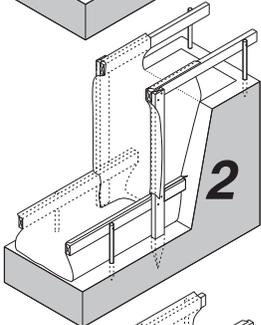
Install the upper level fabric with an 10" overlap. Cut the overlap on the footing width line, letting center portion hang down bank.
