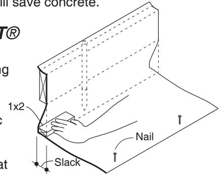
Provide some slack in the fabric by using a 1x2 as shown to prevent excessive downward pressure. Nail fabric to ground at 4' centers to stop fabric pull-out from concrete pressure. Allow an 10" overlap on all joints.
