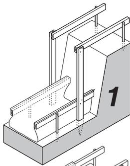
Run fabric up bank to form step. Most steps are too deep to form with a single fabric width. Either run two widths of fabric as edging or turn the fabric 90 degrees to obtain the required width.
