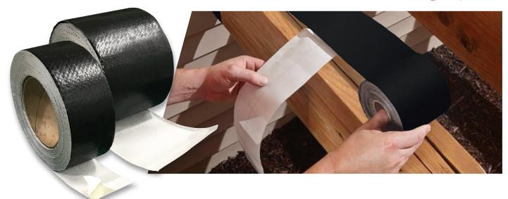
A self-adhering, cold-applied tape used as flashing on deck ledger boards and joists without the need for a primer DECK JOIST TAPE is a self-adhering, cold-applied tape used as flashing on deck ledger boards and joists to help prevent moisture penetration around properly installed fasteners.
